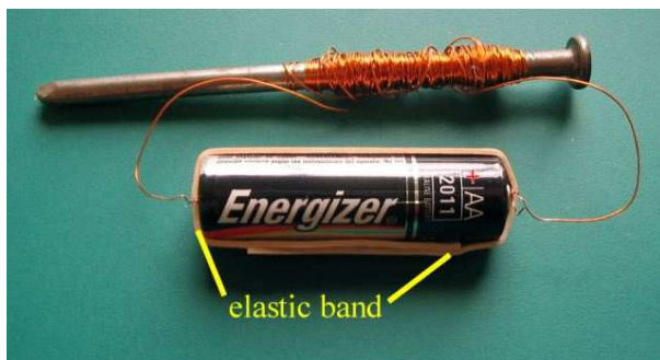
Figure 6: The current carrying copper wire in the above figure creates a magnetic field in the metallic nail.
